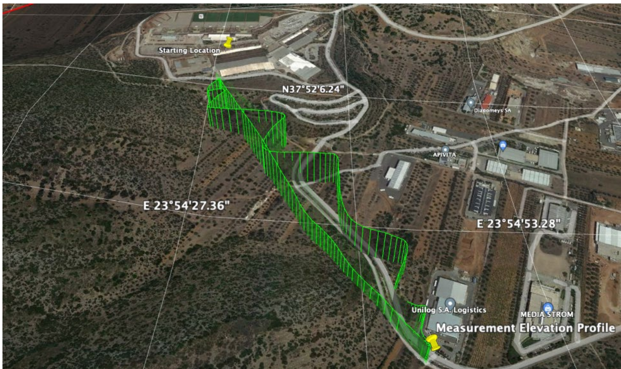
Figure 50 — Zig-zag flight paths of a DJI 210 RTK during a test on 8th March 2023 in the first trial used as ground truth for the DTI systems performance evaluation
