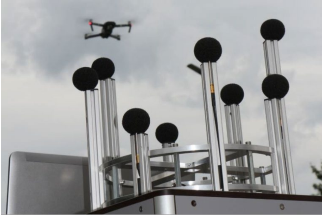
Figure 20 — AMBOS acoustic drone detection system developed at the Fraunhofer Institute, https://www.fkie.fraunhofer.de/en/departments/kom/ambos.html#1514342531
